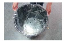
5. Place a new dustbag in the dirt container. Pull the dustbag fastener far enough over the edge of the dirt container so that the dustbag protrudes 2 centimetres over. The pull string should point straight forward. Pull carefully on the strings till the external edge of the dustbag is tight against the dirt container.
