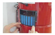
1. Push down the grid of the carbon filter.
