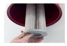
5. Re-insert the filter once it has been fully airdried. Push the filter over the filter holder and tighten the screws.
