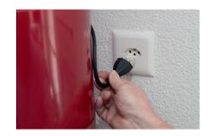
10. Insert the plug again. The Reset button on your **profivac IntelligentSystem** device must then be pressed for at least five seconds to clear the maintenance displays. Your device is now ready for operation again.
