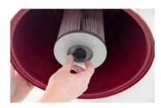
2. Loosen the screws and pull the filter out of the filter holder.
